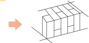
The beams for the roof also share a common interlocking detail, the vertical post taking on the loads from the two beams it supports.
