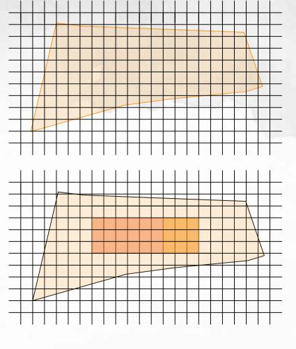
The site is divided with a squared net with sides of 2meters. We created a rectangle and divided it into two parts for two different functions and took out the volume that was needed for the functions of the pavilion.
