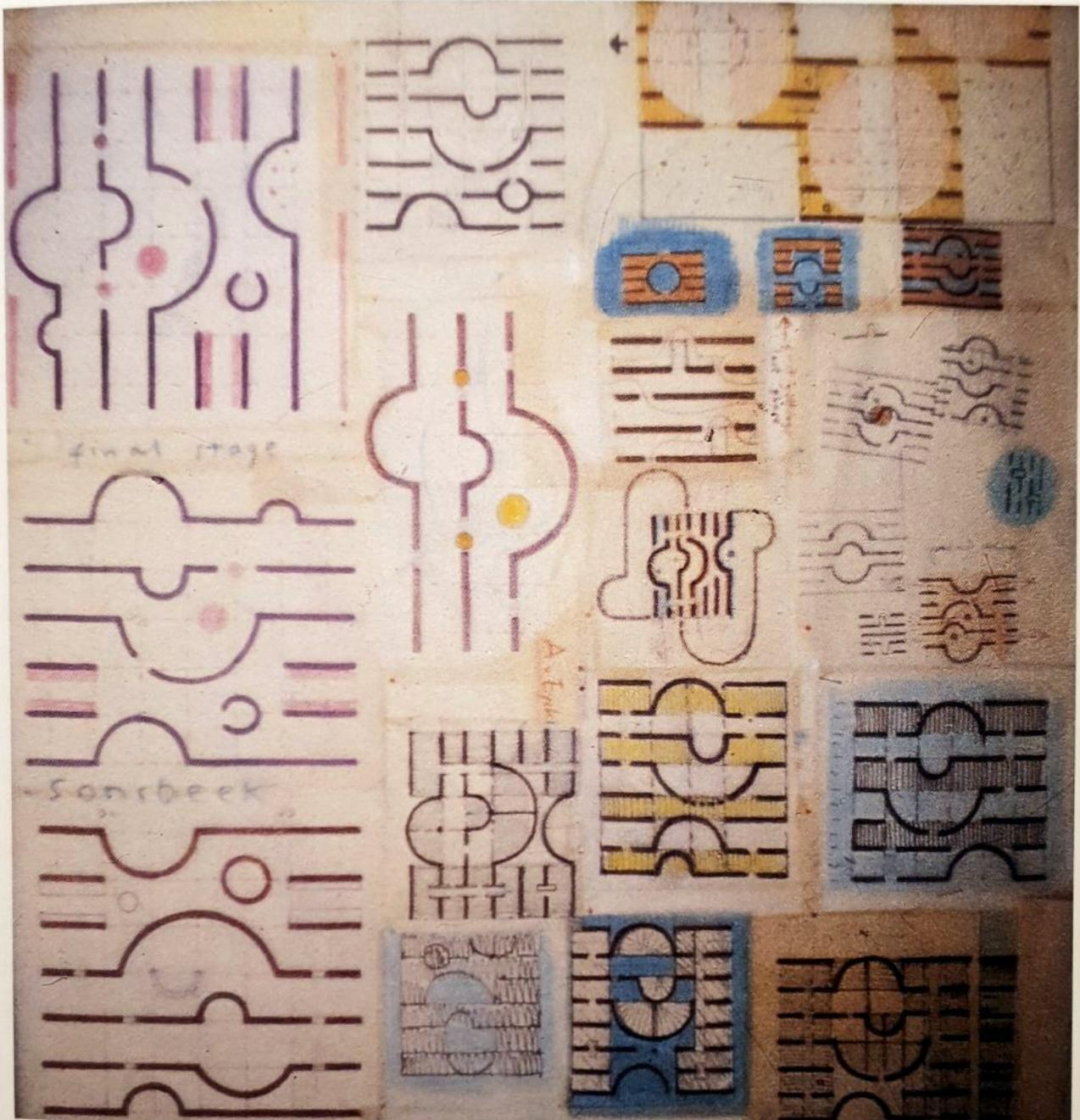
Since the building was intended to be temporary, Van Eyck initially saw it as a light-weight construction of rush mats supported in a wooden framework, the whole of which was to be sprayed with silver paint, as was the large circle in which it stood: a structure made of denaturalized organic material in the middle of the park. As this idea proved difficult to implement in the short term, he opted for a construction in B2-sized concrete blocks.
